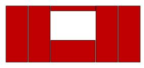
6.4m wide x 2.7m high felt covered stage set with 8' x 4'6 (16:9) central rear projection screen, including braces, stage weights and clamps.
